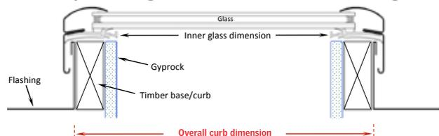
Note: If timber hob is greater than 38mm the Gyprock will encroach on the glazing area.
