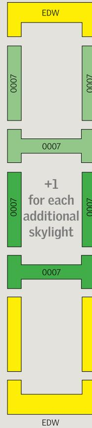
Select your skylight configuration and note the flashing components required.
